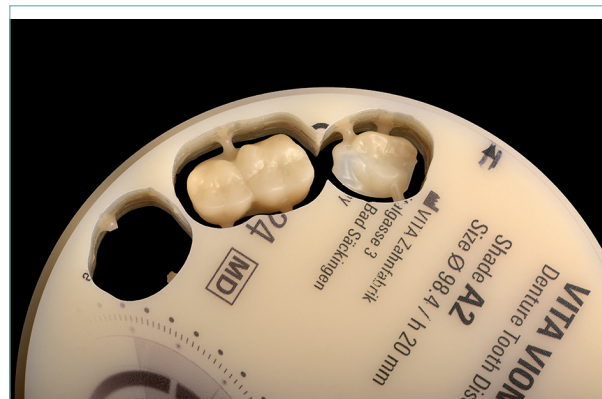
The dental material fabricated with CAD/CAM support in VITA VIONIC DENT DISC multiColor.
